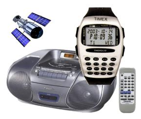
An embedded computer is designed for and built into a specific application where it will perform a limited range of dedicated functions. The size and functionality of an embedded computer depends on the application. They may be very small devices built into a single microchip and may control.
