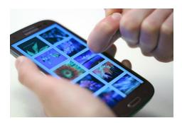
A touch screen is a two way user interface. It is both an input and output device. You can interact with the computer by touching pictures or words on the screen. Touch screens are widely used with tablet PCs, PDAs and smart phones.
