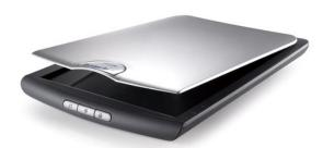
A scanner reads printed data into the computer. A number of different devices are referred to as scanners:
