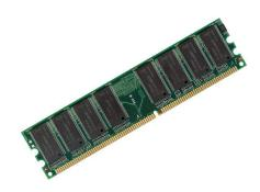
Random access memory can be written to, read from and edited. The data in it can be accessed in any order. Ram is volatile memory, which means that it is cleared when the computer is switched off.
