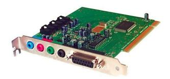
A sound card controls all input and output of audio. Audio input through a microphone and output through speakers are usually analogue and the sound card handles their conversion into digital signals processed by the computer. It also handles digital audio input, e.g. from multimedia applications.
