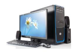
A desktop PC usually has these basic components: a monitor, a keyboard, a system unit and a mouse.
