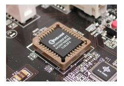
Read only memory can also be accessed in random order, but the data in it cannot be changed. ROM is intended for permanent data, necessary for the operation of the computer system. ROM is non-volatile, which means that it retains what is stored in it when the computer is turned off. *Types of ROM:*
